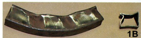
Single Pass 20" I.D. Profile Collapse
