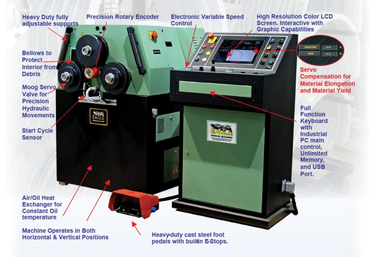
The EAGLE-BPR BA50CNC is a three driven rolls bending machine driven by a sophisticated but easy to use computer program.
